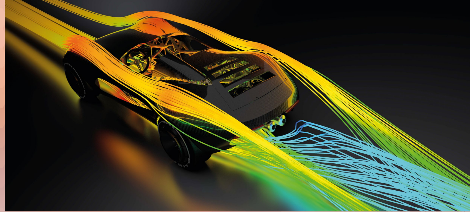
Hack Rod hopes to be the first generatively designed, 3D-printed car. A hot-rod chassis was scanned and digitised, and imported as a 3D model into a computer that produced many design options before printing
